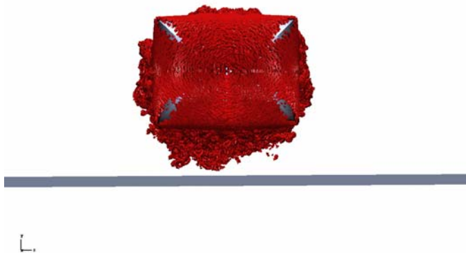
Figure 19. Front view of vortices in Ahmed body flow.
