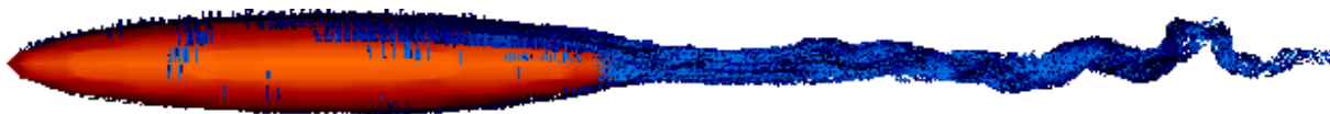
Figure 4: Typical vortex filament structure of the turbulent separated flow past a 6:1 prolate spheroid at 0^\circ angle of attack and R = 4.2 \cdot 10^6 . Vortex elements are drawn as cylinders. Side view.
